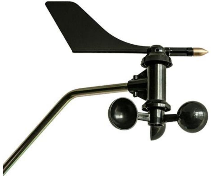
**WAM-1**, uses a three cup anemometer for high accuracy, sensitivity and durability. The cups are connected to a shaft which turns a sensing element that converts the rotation into a series of electronic pulses.
