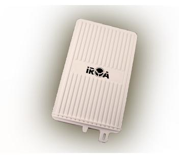
IPM 05 is microcontroller based prepaid energy meter which is especially designed for solar ac micro grids. It has 5 channels and each of them can be programmed separately for desired watt hour credit, watt limit and number of days .Multi channel design allows to connect 5 different households using a single meter but measuring usage of individuals at same time.
